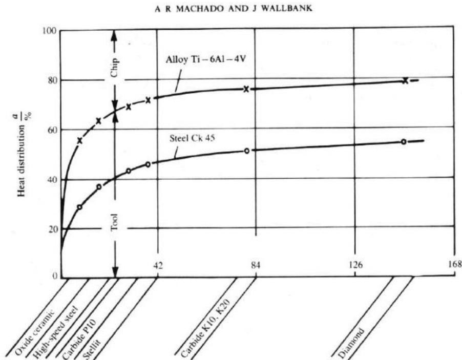
Figure 2 - Distribution of heat generated when machining titanium and steel (after König<sup>3</sup>)
