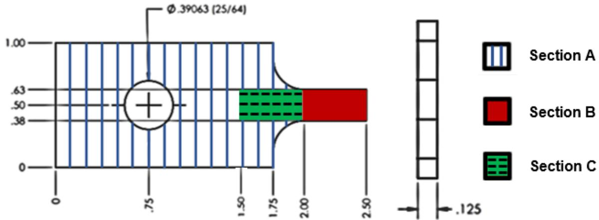
**Figure 1.** Sample dimensions, in inches, for all materials used. Different Sections are separated to be sanded and treated in all experiments.
