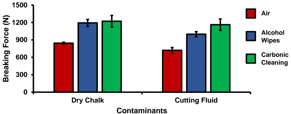
**Figure 10.** Breaking force (N) measured after force-tester analysis for surface pretreatments of air (red), alcohol wipes (blue), and Carbonic Cleaning (green) on Aluminum to ABS surfaces after sanding with dry chalk and cutting fluid contaminants.
