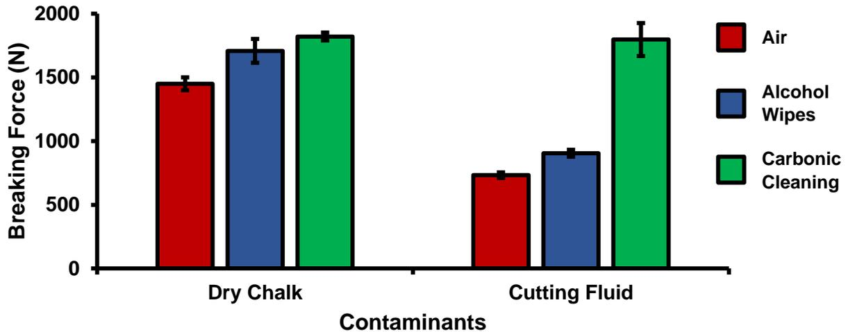
**Figure 6.** Breaking force (N) measured after force-tester analysis for surface pretreatments of air (red), alcohol wipes (blue), and Carbonic Cleaning (green) on Aluminum to Aluminum surfaces after sanding with dry chalk and cutting fluid contaminants.
