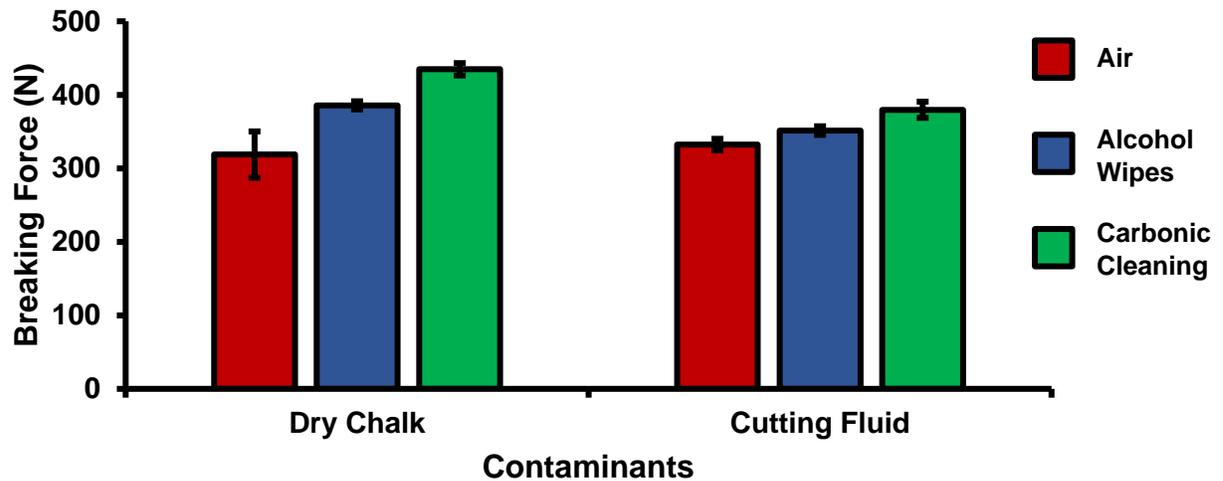
**Figure 8.** Breaking force (N) measured after force-tester analysis for surface pretreatments of air (red), alcohol wipes (blue), and Carbonic Cleaning (green) on ABS to ABS surfaces after sanding with dry chalk and cutting fluid contaminants.
