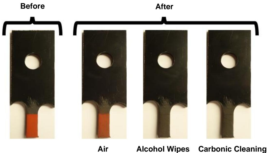
**Figure 5.** ABS samples with dry chalk applied before cleaning (far left), after air pretreatment (middle left), after alcohol wipe pretreatment (middle right), and after Carbonic Cleaning pretreatment (far right).
