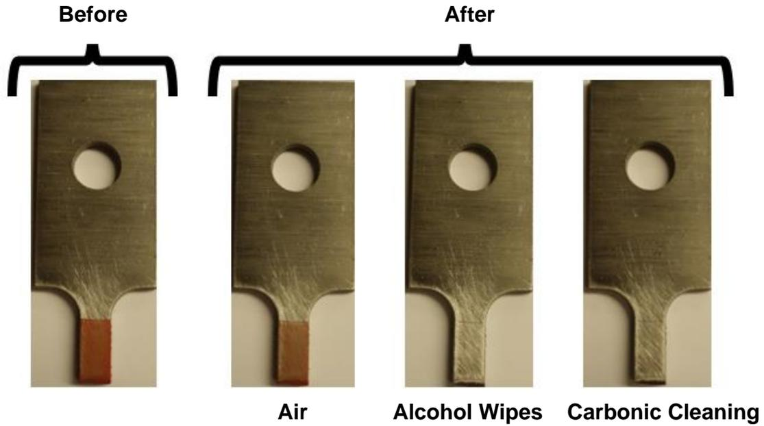
**Figure 4.** 304 Stainless Steel samples with dry chalk applied before cleaning (far left), after air pretreatment (middle left), after alcohol wipe pretreatment (middle right), and after Carbonic Cleaning pretreatment (far right).
