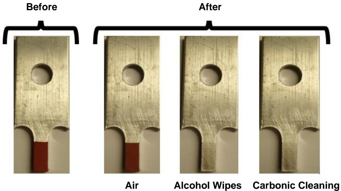
**Figure 3.** 6061 Aluminum samples with dry chalk applied before cleaning (far left), after air pretreatment (middle left), after alcohol wipe pretreatment (middle right), and after Carbonic Cleaning pretreatment (far right).
