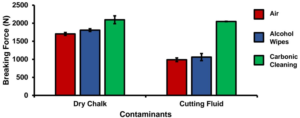
**Figure 9.** Breaking force (N) measured after force-tester analysis for surface pretreatments of air (red), alcohol wipes (blue), and Carbonic Cleaning (green) on Aluminum to Stainless Steel surfaces after sanding with dry chalk and cutting fluid contaminants.
