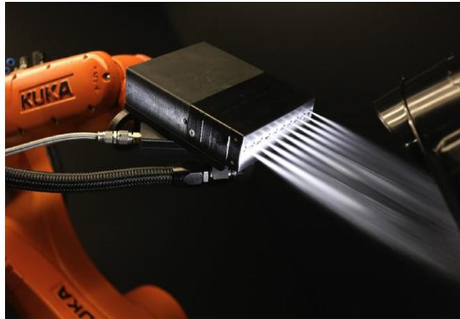
FIG. 3: M2 Cleaning Effector with CO<sub>2</sub> Streams
