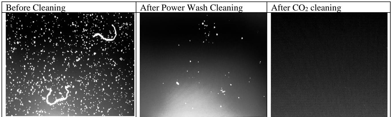
FIG. 6 Partsens Microscope Particle Counter images before after supercritical CO<sub>2</sub> cleaning
