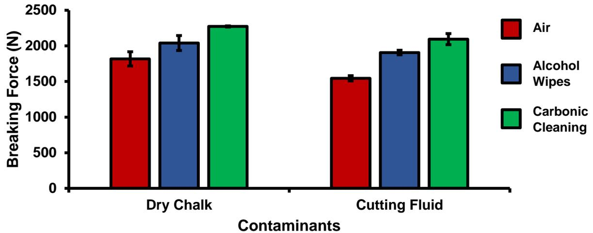
**Figure 7.** Breaking force (N) measured after force-tester analysis for surface pretreatments of air (red), alcohol wipes (blue), and Carbonic Cleaning (green) on Stainless Steel to Stainless Steel surfaces after sanding with dry chalk and cutting fluid contaminants.
