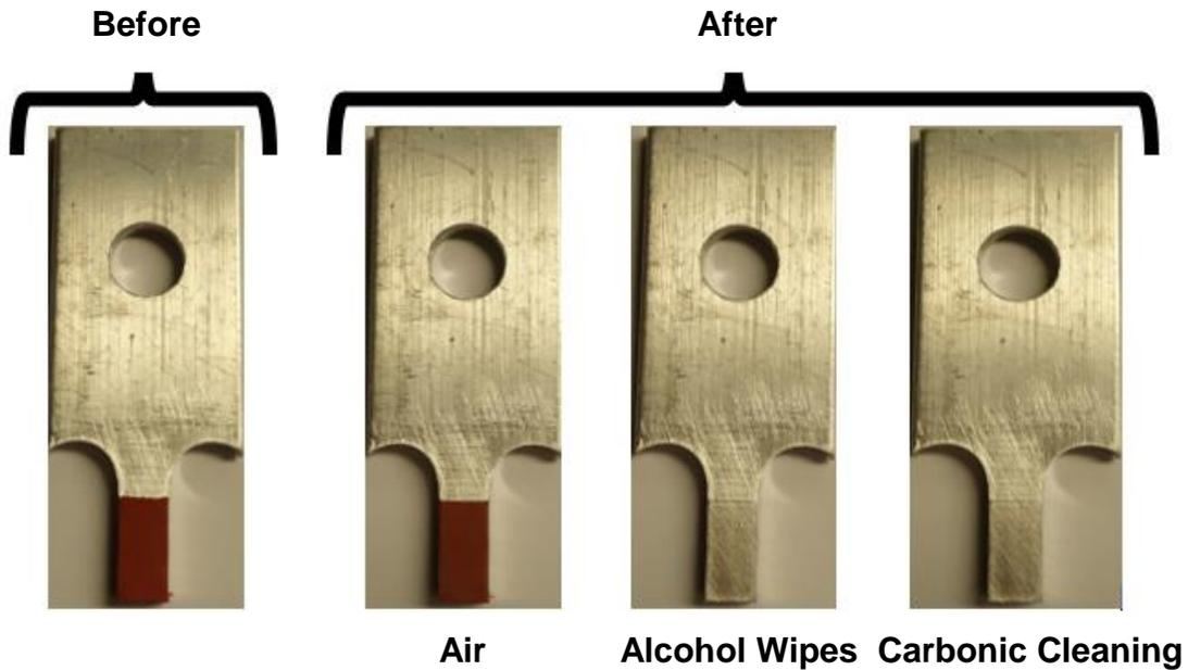
**Figure 3.** 6061 Aluminum samples with DeWALT level 4 dry chalk applied before cleaning (far left), after air pretreatment (middle left), after alcohol wipe pretreatment (middle right), and after Carbonic Cleaning pretreatment (far right).
