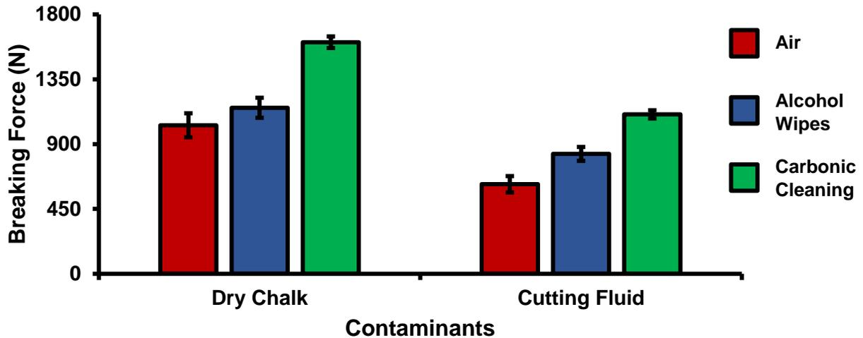
**Figure 11.** Breaking force (N) measured after force-tester analysis for surface pretreatments of air (red), alcohol wipes (blue), and Carbonic Cleaning (green) on Stainless Steel to ABS surfaces after sanding with dry chalk and cutting fluid contaminants.
