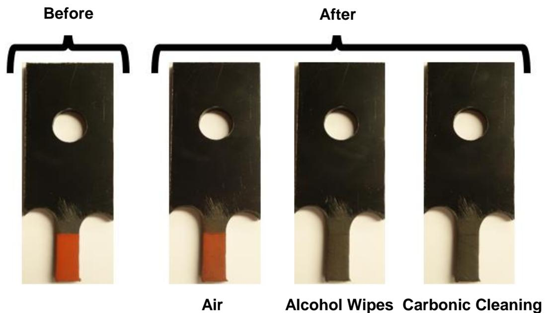
**Figure 5.** ABS samples with DeWALT level 4 dry chalk applied before cleaning (far left), after air pretreatment (middle left), after alcohol wipe pretreatment (middle right), and after Carbonic Cleaning pretreatment (far right).
