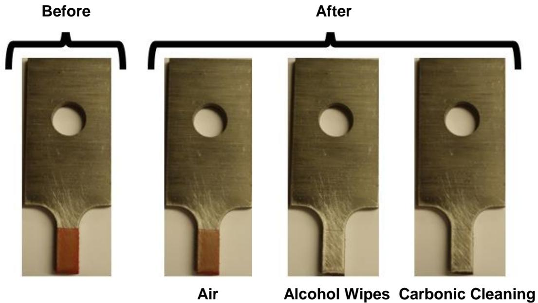
**Figure 4.** 304 Stainless Steel samples with DeWALT level 4 dry chalk applied before cleaning (far left), after air pretreatment (middle left), after alcohol wipe pretreatment (middle right), and after Carbonic Cleaning pretreatment (far right).
