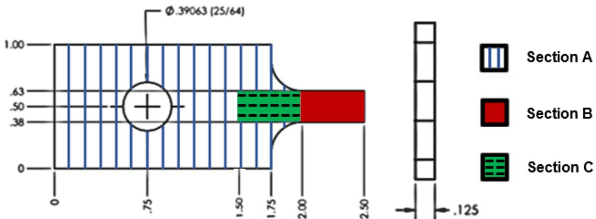
**Figure 1.** Sample dimensions, in inches, for all materials used. Different Sections were separated to be sanded and treated in all experiments.
