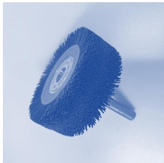
to these brushes is that they are extruded from nylon and other forms of thermal-melt polymers. When used without coolants, excessive speeds and feeds can cause the brushes to melt or otherwise lose their shape.
